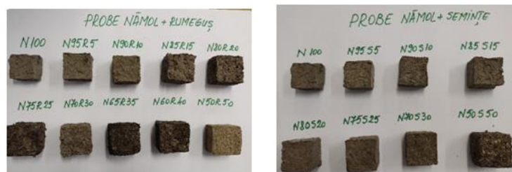
Fig. 5. 48. Composite Material Samples Two Weeks After Removal from the Forming Mold.
