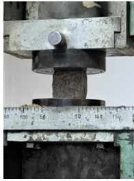
Fig. 5. 67. Positioning and Alignment of the Specimens on the Mechanical Testing Machine Support
