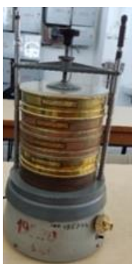
Fig. 5.3. Vibratory Screening Apparatus
